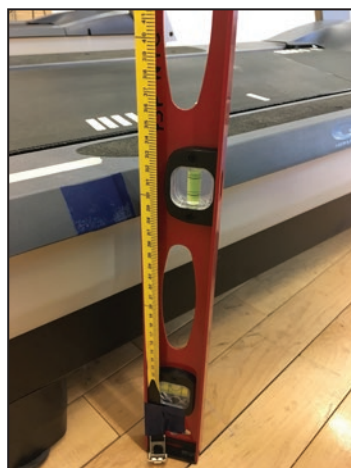
Figure 34: Measure the height at each end of the 1 m
