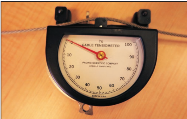
Figure 47: Cable installed properly with trigger closed
