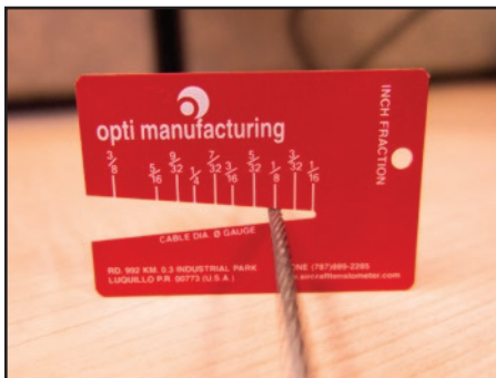
Figure 40: Tool to measure the size of your cable
